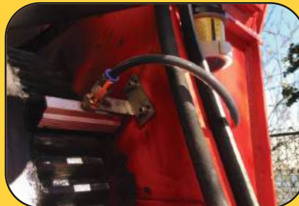
Open Gears – Brush application
