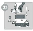
Install the base on the bracket using a strong threadlocker.
