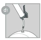
Prime lube point and remove nipple.
