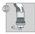
Screw tightly keeping the assembly aligned.
