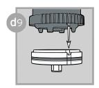
Insert the pin of the module into the notch of the base.
