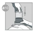
Screw tightly keeping the assembly aligned.
