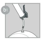
Prime lube point and remove nipple.
