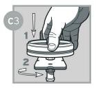
Install the base and F1/4 fitting using a strong threadlocker.
