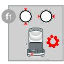
Alternating red light for 1s, every 1os: Gearbox broken or blocked. VISIO stops after 3 trials.
