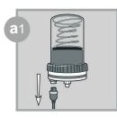
For EP/CONNECT: Disconnect the power plug.
